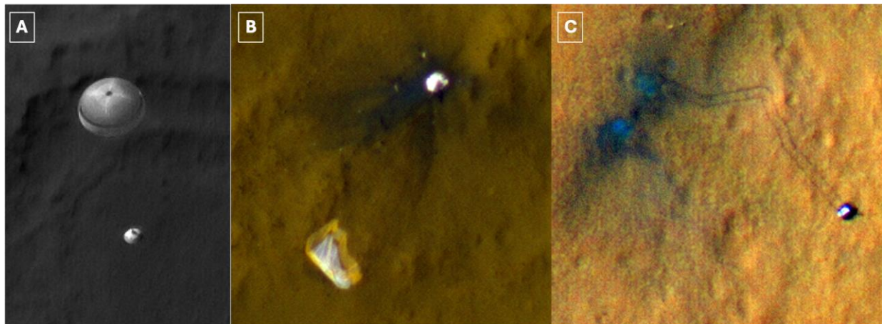
Figure 3. HiRISE subset images of the Entry Descent and Landing (EDL) and first significant traverse of the Mars Science Laboratory "Curiosity" rover. (A) Shows the encapsulated rover while descending through the atmosphere on the parachute and about a minute before touchdown. The parachute is ~16 m in diameter. The parachute and rover were captured in HiRISE image ESP_028256_9022. The intention was to capture this image in colour, but the descent occurred further downrange than expected. If full-swath colour imaging had been possible (as proposed for HRMI), this image would have been in colour. Notably, this image was taken at a high emission angle and phase (almost 45° and over 90°, respectively). (B) Subregion of HiRISE IRB image ESP_028612_1755 showing the final resting place of the parachute and backshell on the surface. (C) The first extended traverse of the Curiosity rover ~4 weeks after landing. The rover is ~3 m wide. Rover tracks, while smaller than the pixel scale of HiRISE, are resolved due to their high contrast with the surface; likewise, the shadow of the mast and its suite of cameras atop the rover can also just be resolved. Credit: NASA/JPL-Caltech/Univ. of Arizona.
