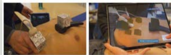
Figure 1: One QR Cube is placed on the ultrasound probe and one on the chest of the subject using a bespoke chest support. The EchoFinder software tracks the QR Cube to save the position and orientation of the ultrasound probe in relation to the reference QR Cube on the chest.
